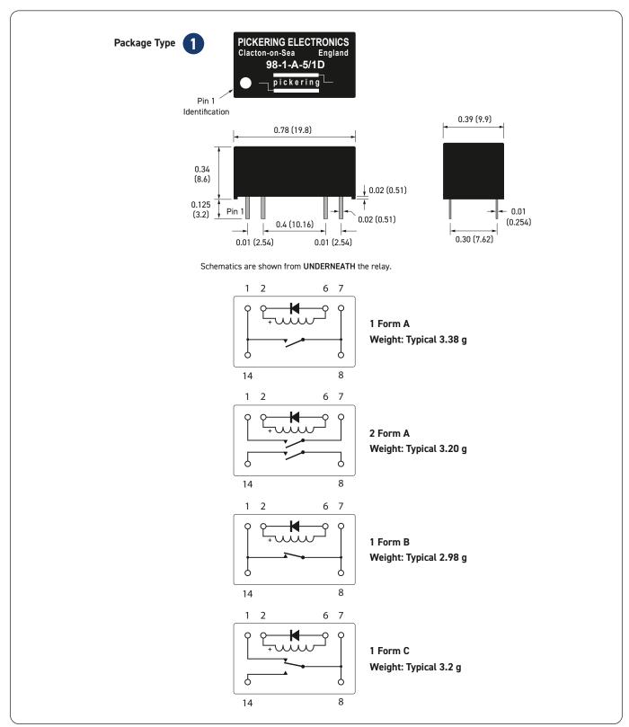
Pin Configuration, Weights and Dimensional Data (dimensions in inches, millimeters in brackets)
